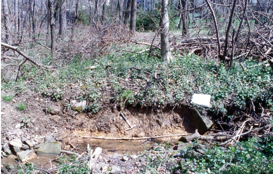
Sta 975 upslope of the eroded ravine – overall of slackwater soil at approximate el. 1116 ft.
