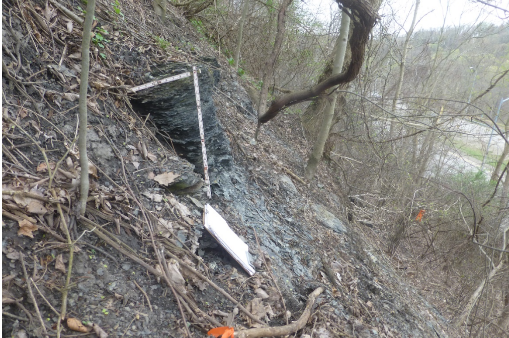
Slumped carbonaceous shale above the Duquesne coal level at approximately 50 ft. south of the eroded ravine.
