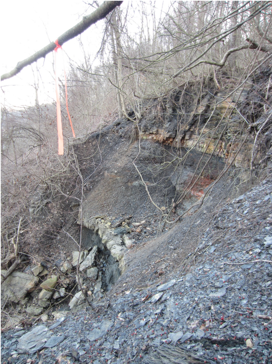
View north at the upper part of the eroded ravine, Ames Limestone up to Duquesne coal – strata dip 7° into the slope – apparently slumped.
