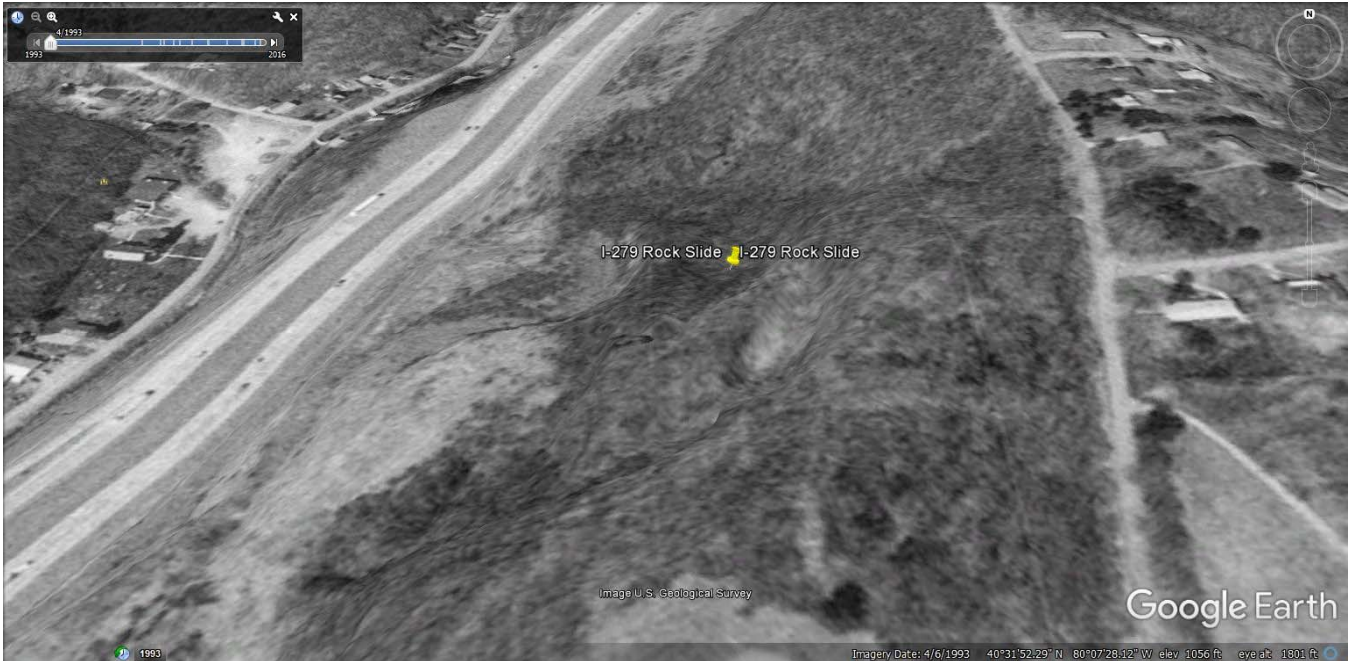
Google Earth photo looking north at the slide area, approximate Sta 902-910. The graben is on the right and below the yellow tack.
