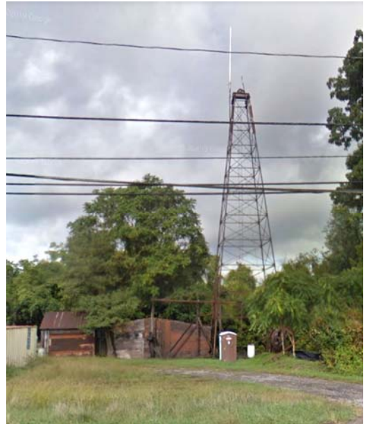
Figure 71. Photograph of an old pipe rig originally drilled on the Jane Riddle lease, date unknown. The current operator is Raymond D. (Ray) Langer, an independent oilman from Coraopolis who established his company in 1964. This well, currently called the Langer #2 Riddle well, produces from the Upper Devonian Venango Group, probably the Fifth sand, at 2,386 feet. This well is in the Moon Run-Crafton oil field, part of the McDonald oilfield complex.
