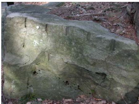
Figure 43. Photograph of a block of Mahoning sandstone at the Allegheny Portage Railroad National Historic Site, showing a stonemason's drill holes. Part of this boulder must have been used on the Portage Railroad as a "sleeper" or an ashlar block.
