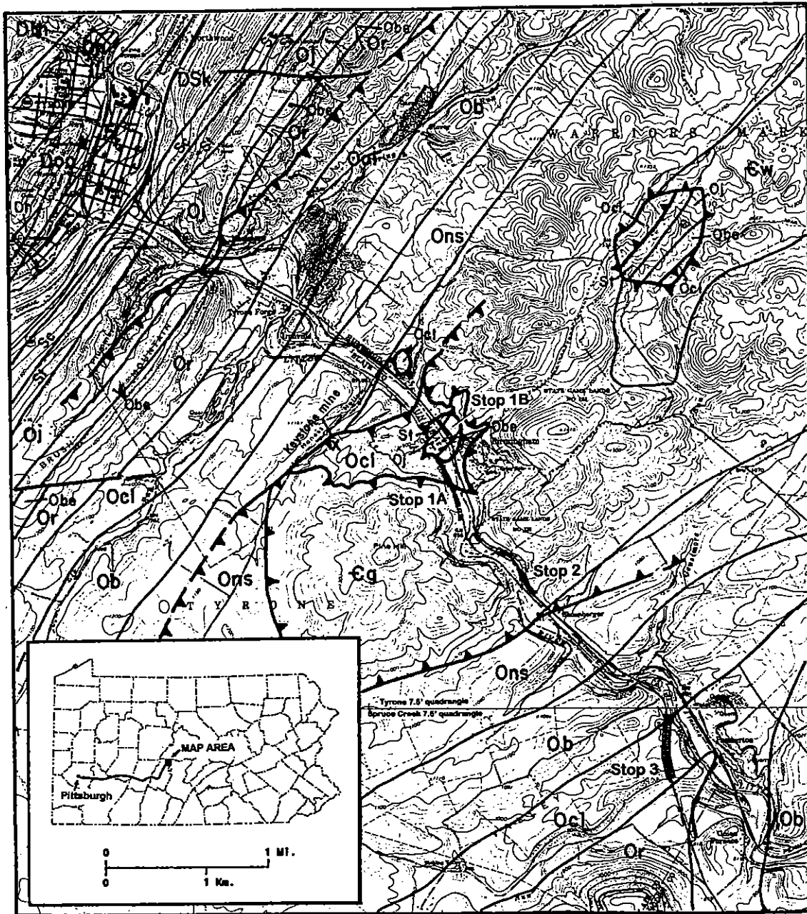
Figure 1. Geologic map of the Tyrone area showing the locations of field stops. Formation abbreviations are as follows: Dbh - Brallier and Harrell formations; Dh - Hamilton Group; Doo - Onondaga through Old Port formations; Dsk - Keyser through Mifflintown formations; Sc - Clinton Group; St - Tuscarora Formation; Oj - Juniata Formation; Obe - Bald Eagle Formation; Or - Reedsville Formation; Ocl - Coburn through Loysburg formations; Ob - Bellefonte Formation; Ons - Nittany through Stonehenge formations; Cg - Gatesburg Formation; and Cw - Warrior Formation.
