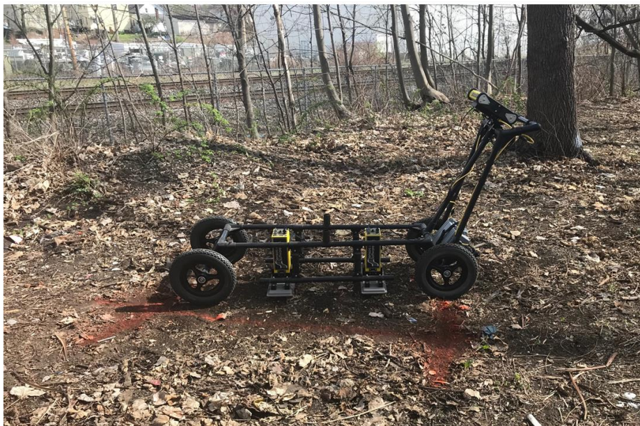
Photograph of YSU's ground penetrating radar device overlying a suspected clandestine grave site at a cold case file crime scene.
