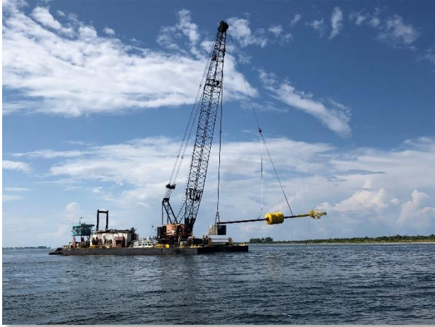
A team from the University of South Florida deploys a buoy off Egmont Key in the Gulf of Mexico that will measure sea floor motion prior to earthquakes and tsunamis.
