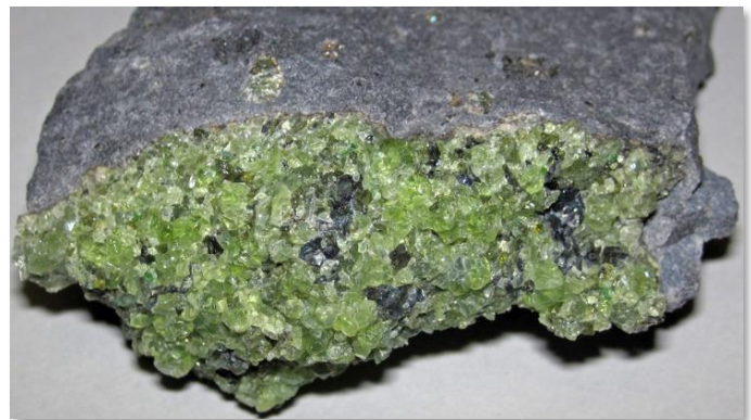
Dunite, an olivine-rich igneous rock, is a promising candidate for long-term storage of atmospheric CO 2 .
